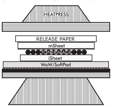
Note: Strip apart right on the heat press in one slow steady motion in an almost horizontal angle!
