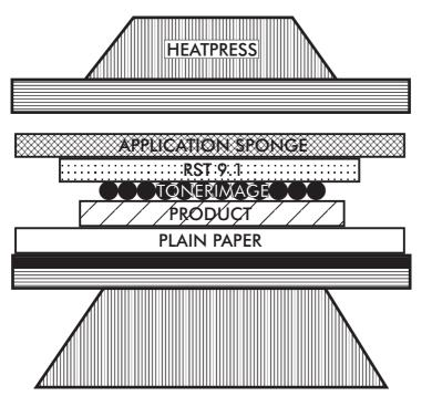
Take product off the HeatPress when finished pressing. Spray the RST paper with water until it completely comes loose from the toner image. Remove RST paper and wipe the image area with a damp/wet towel or cloth.
