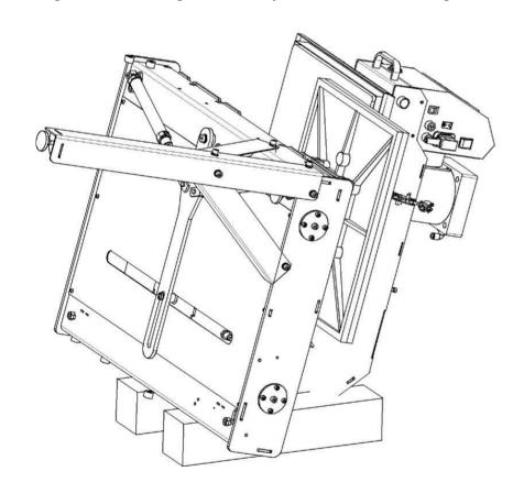
• To do so, use screws (1), washers (2) and spring washers (3). Insert the spacers (5) on the front and the back side of the press.
