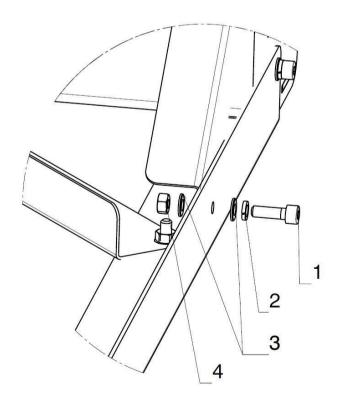
Screw the pneumatic control unit to the press using two screws.
