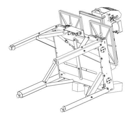
• Carefully position the press with at least 2 persons. In doing so, avoid resting the weight on the rear legs by slightly lifting it off the ground.
