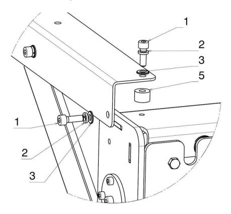
• Screw the stabilizers to the legs using screw (1), washers (3), lock washer (2) and nut (4) from the **inside**.
