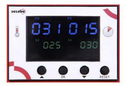
With a large digital controller, temperature (°C und °F) and pressing time can be adjusted. The green digits are showing the theoretical value, the white digits are showing the actual value. A counter (at the right bottom) counts the number of transfers that have already been made during the current session. The counter can be reset at any time.
